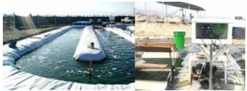
Figure 2. Spirulina pond (left) and the CO2 injection system (right)
