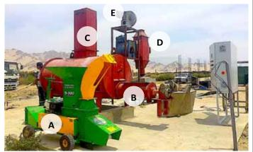
Figure 5. Integrated system from a pyrolyser of continuous production of fertilizers and spirulina. In the image the following phases are described (A) Biomass crusher, (B) entry of organic waste, (C) chimney for the conduction of gases, (D) exchanger for the recycling of heat for the drying of the microalgae and (E) use of CO2 for the production of spirulina. Photo: Yngrid Espinoza.
